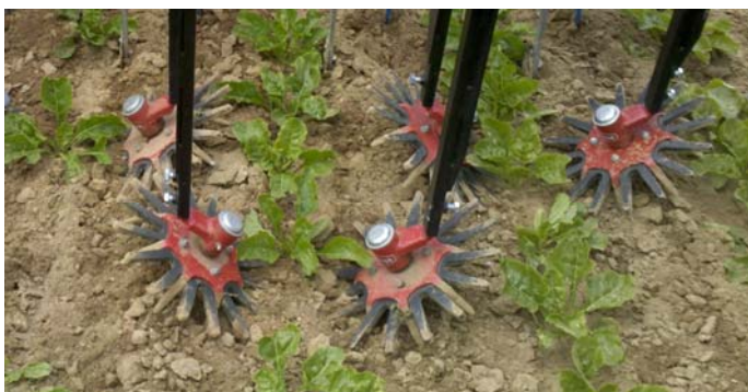
Finger weeder in action: IIRB experts in Agricultural Engineering and Weed Control attended Dés herb'Avenir IV to experience and discuss the potential of mechanical weed control
